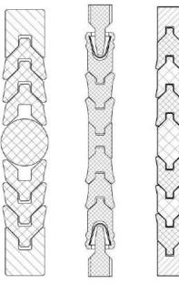
**Seal Stack** is comprising a top adapter or anti-extrusion ring , Vee Rings and a bottom adapter .
