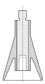
Pump Down Plugs separate cement from the displacement fluid during liner cementing operations.
