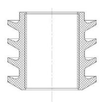
Liner Wiper Plugs separates drilling fluid from cement during displacement. It can reverse in the pipe without breaking the lips. Products can be produced in a variety of compounds and are available in sizes ranging from 3 ½" to 9 5/8".
